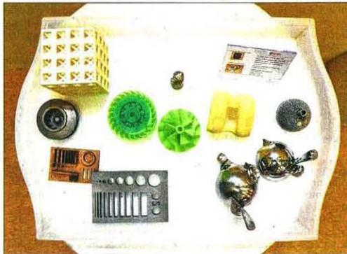
Items made by selective laser melting of steel, cobalt chrome and titanium alloys for biomedical implants at the new NTU Additive Manufacturing Centre.
