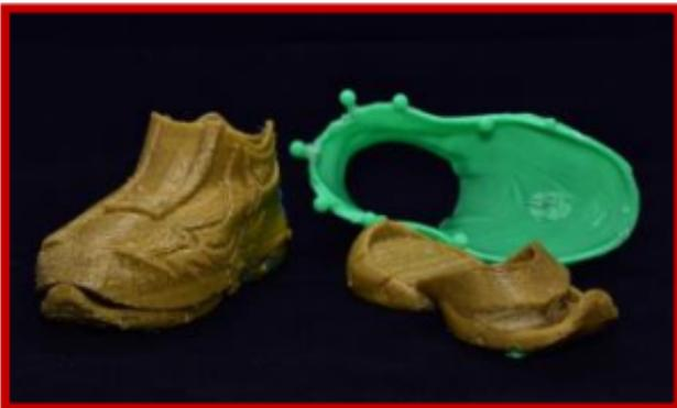
This design is built on the idea that slippers can be constantly upgraded to fit wearer's personality and interests, with changeable casings allowing for diversity on different occasions. Printed using TPU to achieve a soft, cool-dry texture, rectangle blocks with words are glued onto slippers, acting like stamps on ground, allowing for customisation.
