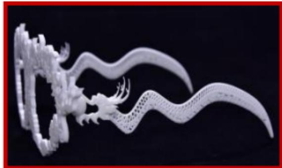
Showcasing the advantage of 3D Printing, the Chinese Dragon consist of nested sphere structures which can not be produced by traditional methods . The front part of design has a spherical curvature to fit the curve of head. The shape of legs is accurately calculated by mathematical function to surround the user's ears comfortably.
